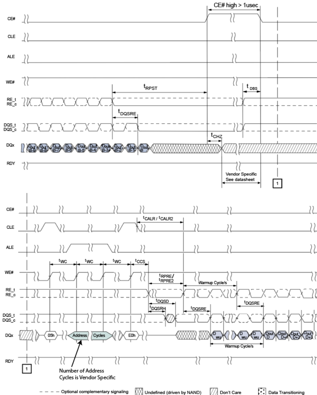
Figure 4-4 Example of Data Output Burst Exit with CE_n High > 1uS and Resume Sequence for Devices that Support greater than 800 MT/s
