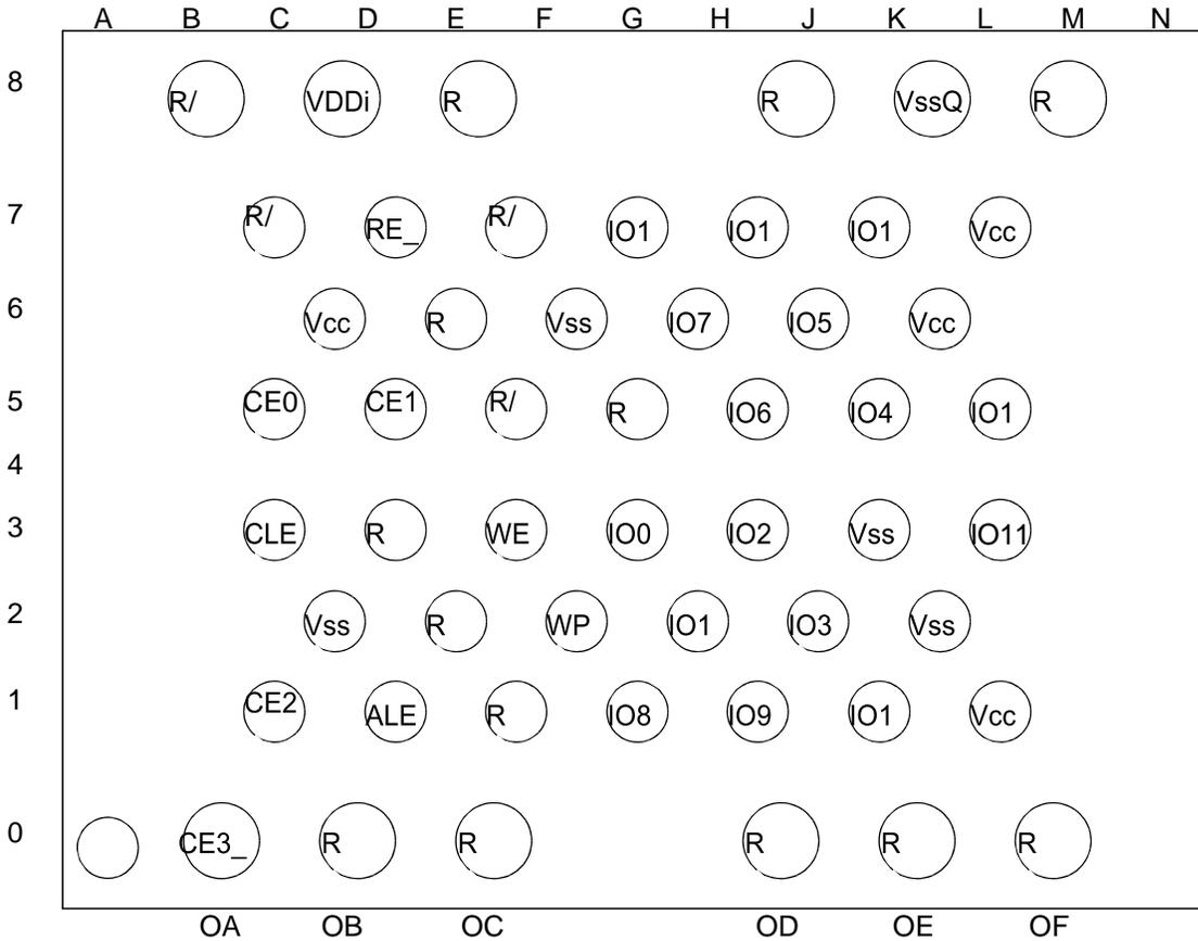
Figure 10 — LGA pinout for 16-bit data access
