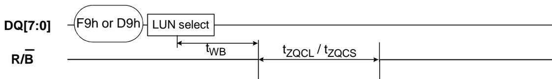
**Figure 24 — ZQ calibration Sequence**
