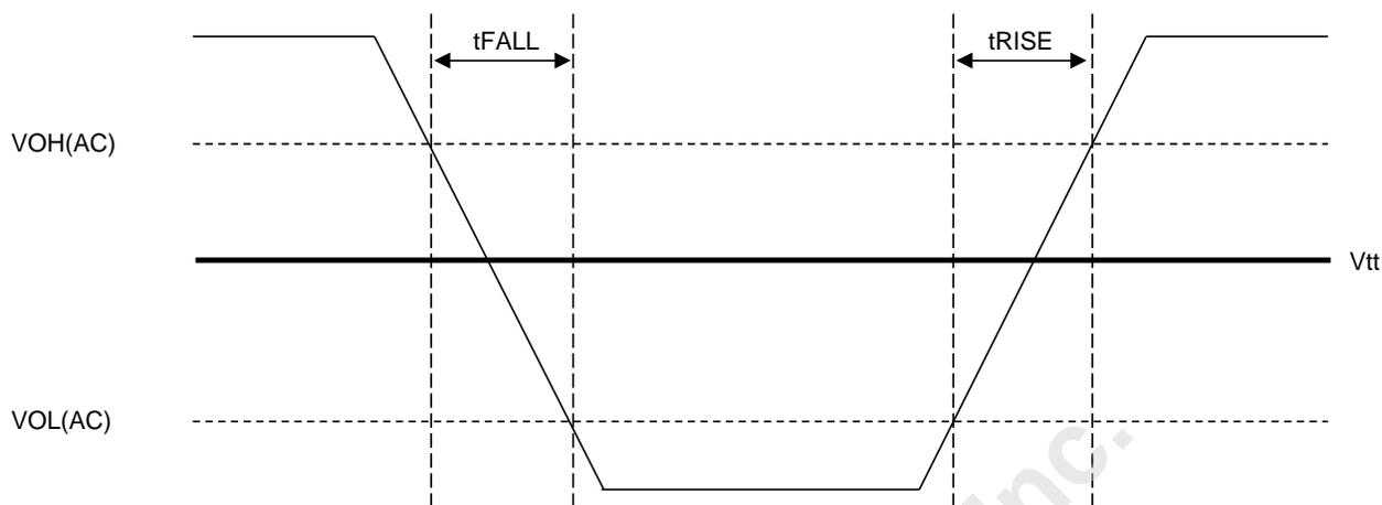
Figure 23 — tRISE and tFALL Definition for Output Slew Rate, (single-ended)
