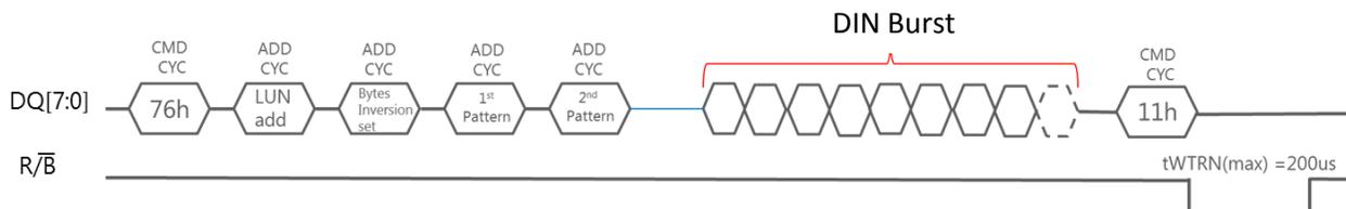
DIN Burst: Data Input with the same pattern specified in 3 address cycle wrapping around the data pattern length (16 or 32) for 1 full page
