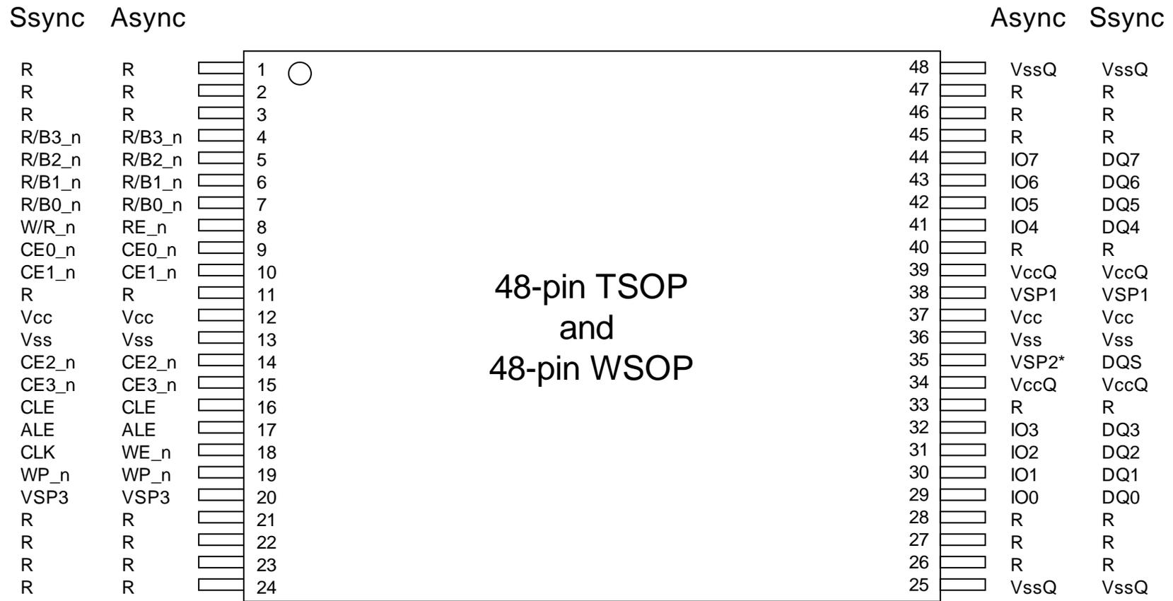
**Figure 2** 48-pin TSOP/WSOP pinout for 8-bit data access
