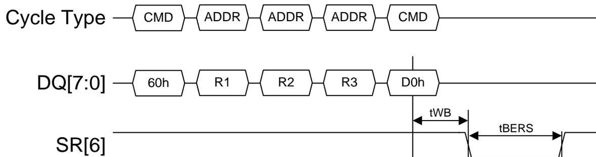
**Figure 5-15 Block Erase timing**
