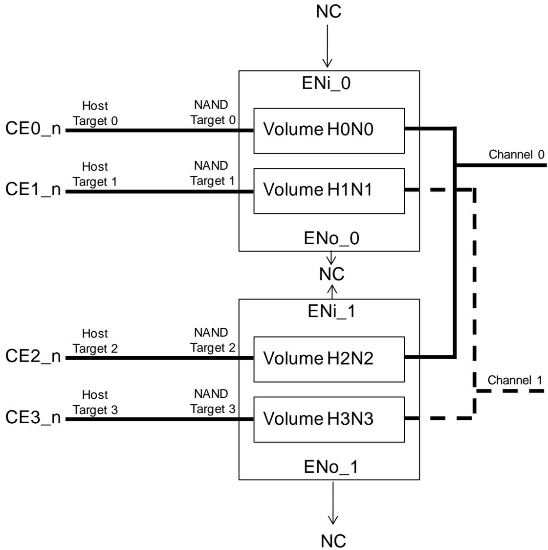
Figure 2-36 Discrete CE<sub>n</sub> per package topology
