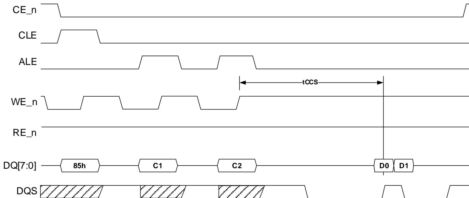
**Figure 5-4 NV-DDR2, NV-DDR3 and NV-LPDDR4 data interface command description**
