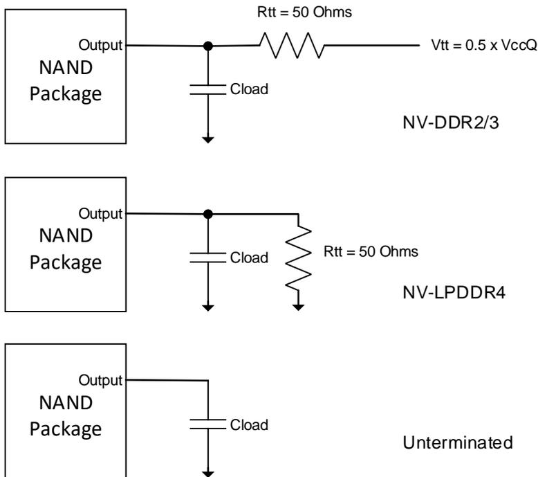
**Figure 4-6 Driver Output Reference Load**
