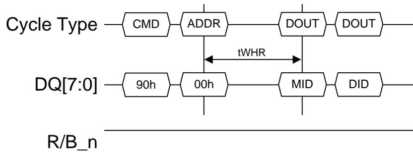
**Figure 5-9 Read ID timing diagram for manufacturer ID**
