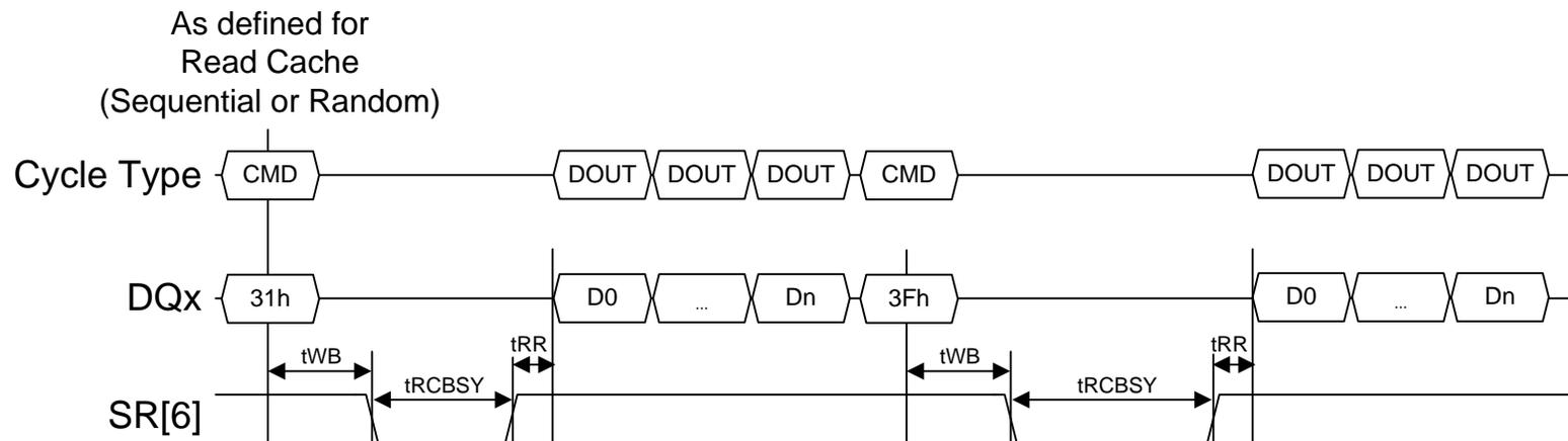
**Figure 5-24 Read Cache timing, end of cache operations**
