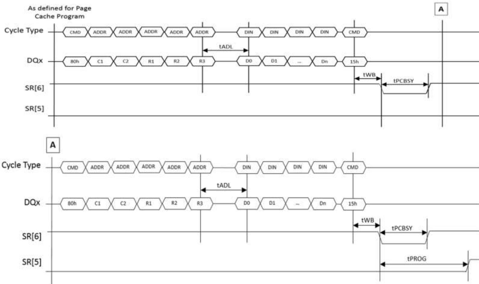
**Figure 5-28 Page Cache Program timing, end of operations using 15h**
