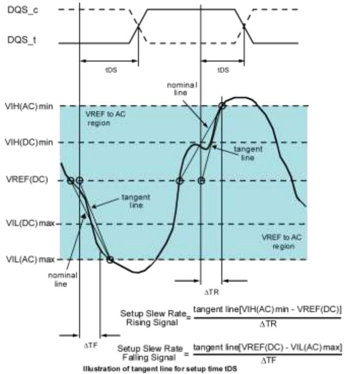
Figure 4-13 Tangent Line for Data Setup Time (tDS)
