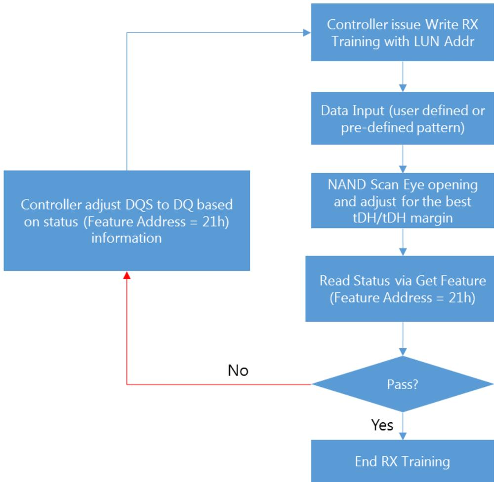
**Figure 5-54 Flow chart for Write DQ Training (Rx side)**
