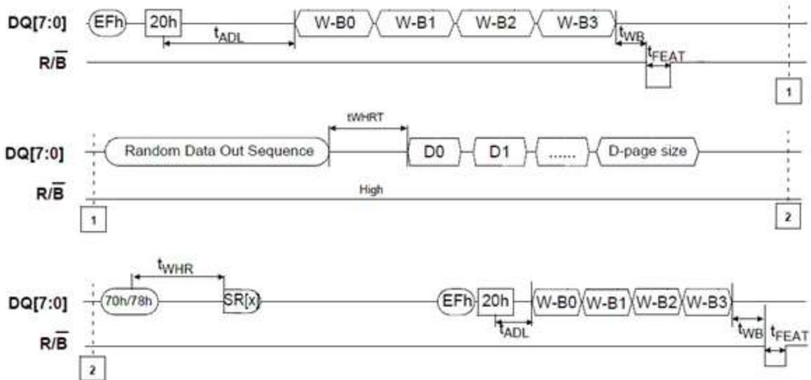
Figure 5-48 DCC (RE\_t/c) Training using Set Feature
