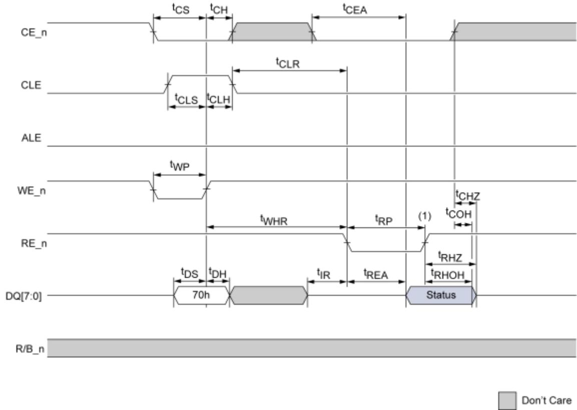
Figure 5-17 Read Status command using SDR data interface
