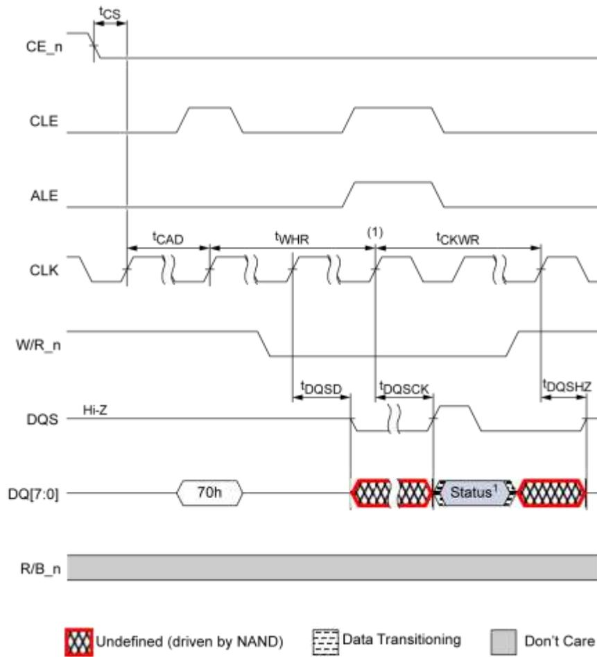
**Figure 5-18 Read Status command using NV-DDR data interface**
