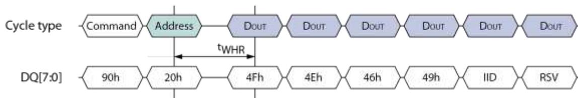
Figure 5-8 Read ID timing diagram for ONFI signature
