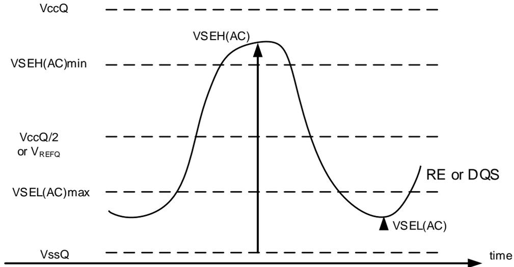
**Figure 2-30 Single-Ended Requirements for Differential Signals**
