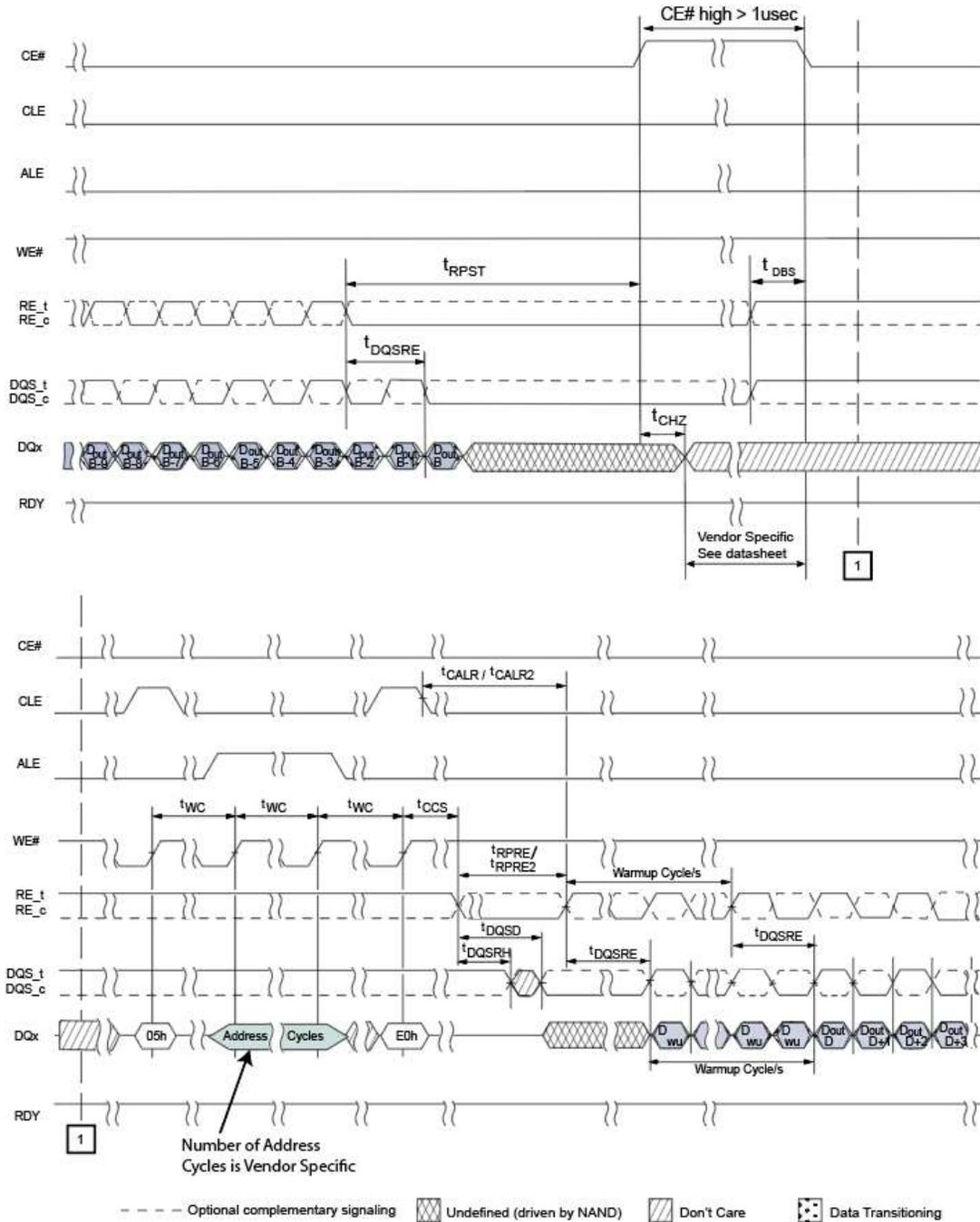
**Figure 4-4 Example of Data Output Burst Exit with CE<sub>n</sub> High > 1uS and Resume Sequence for Devices that Support greater than 800 MT/s**
