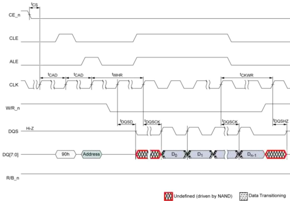
Figure 5-11 Read ID command using NV-DDR data interface
