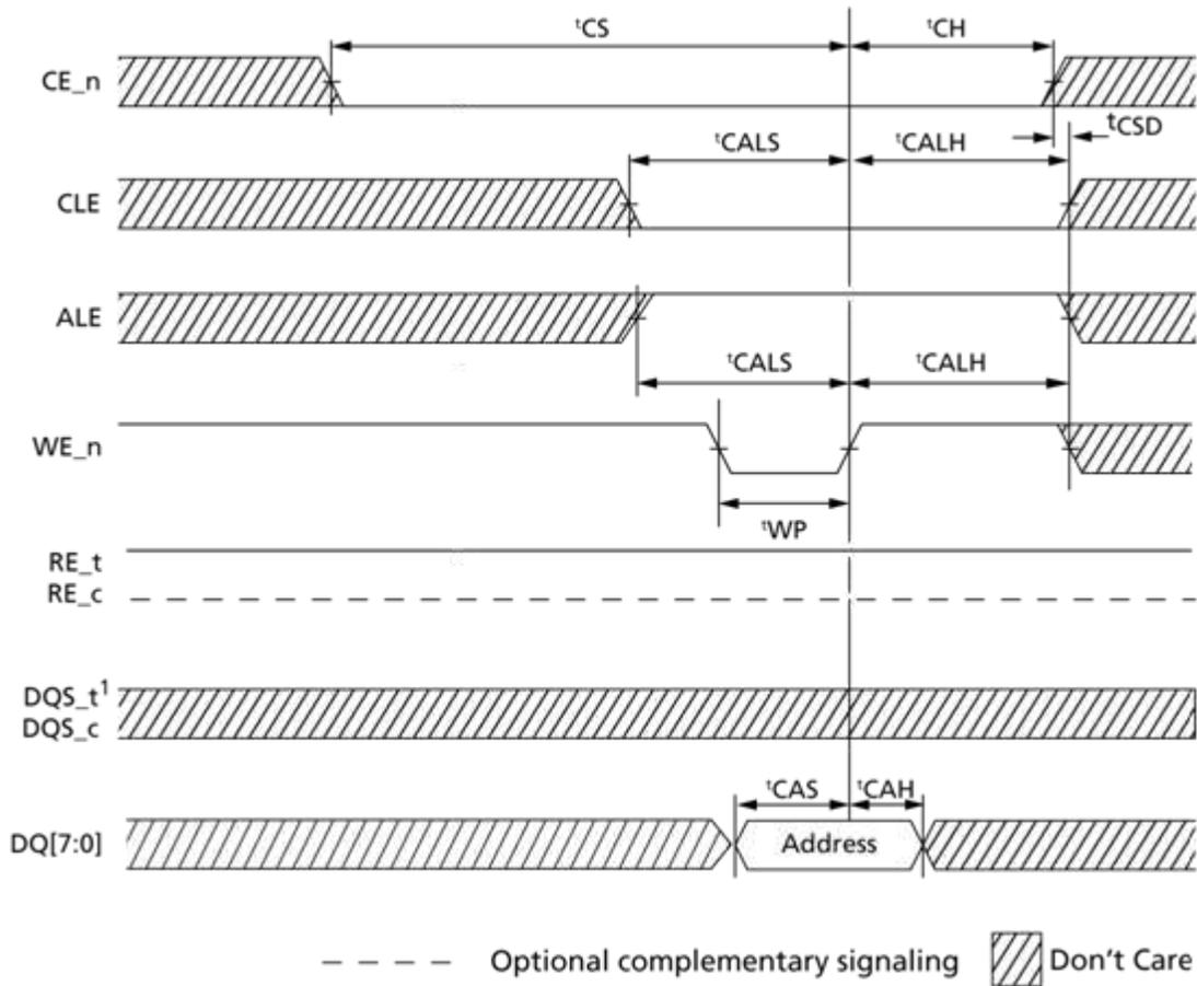
**Figure 4-41 Address cycle timings**
