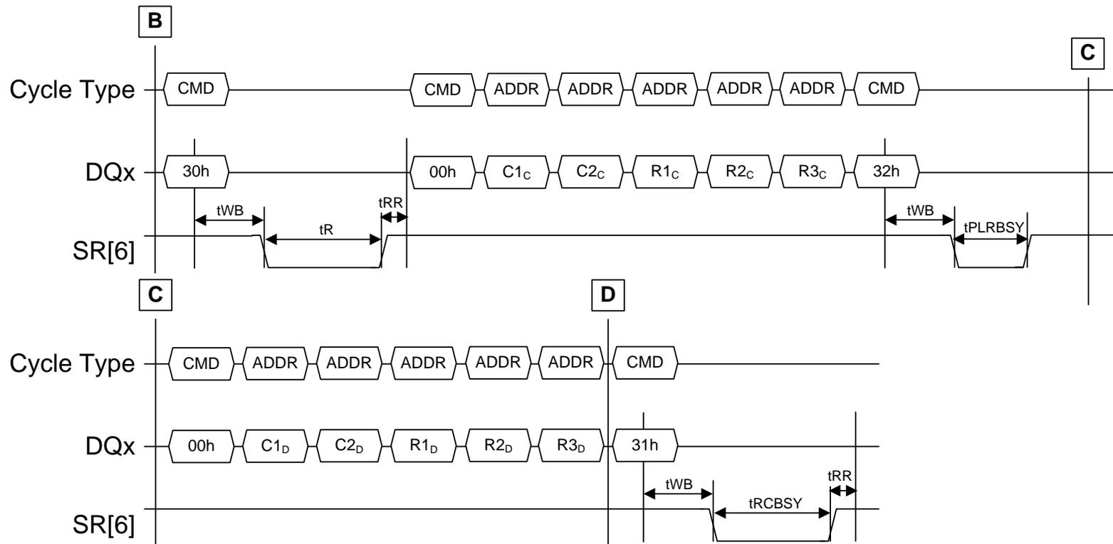
**Figure 6-13 Multi-plane Read Cache Random command issue timing**
