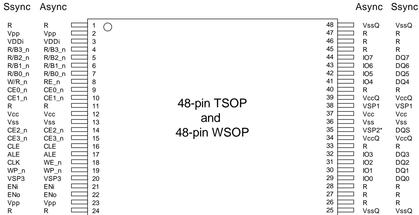
**Figure 2-1 48-pin TSOP/WSOP pinout for 8-bit data access**
