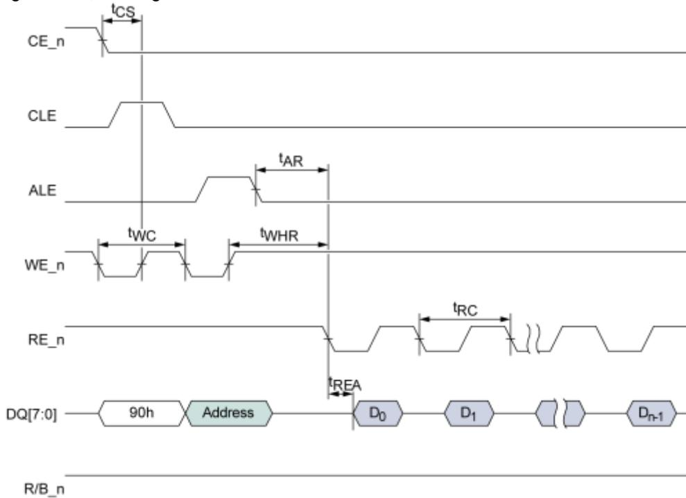
**Figure 5-10 Read ID command using SDR data interface**
