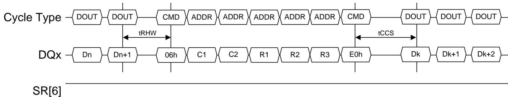
**Figure 5-35 Change Read Column Enhanced timing**
