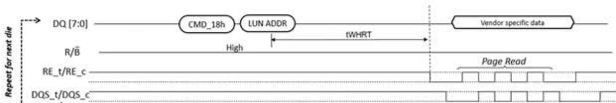
Figure 5-49 DCC (RE\_t/c) Training using Command (Optional)
