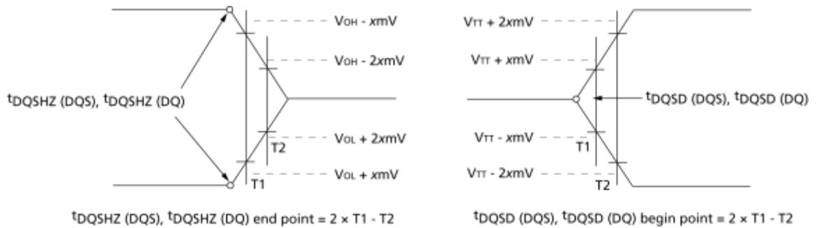
**Figure 7-7 Two point method for measuring timing parameters with tri-state condition**
