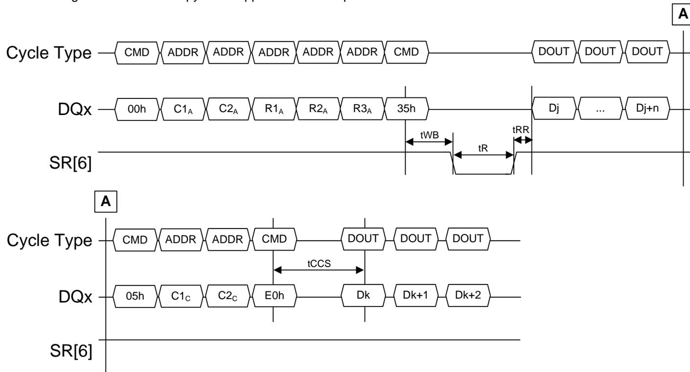
**Figure 5-30 Copyback Read with data output**
