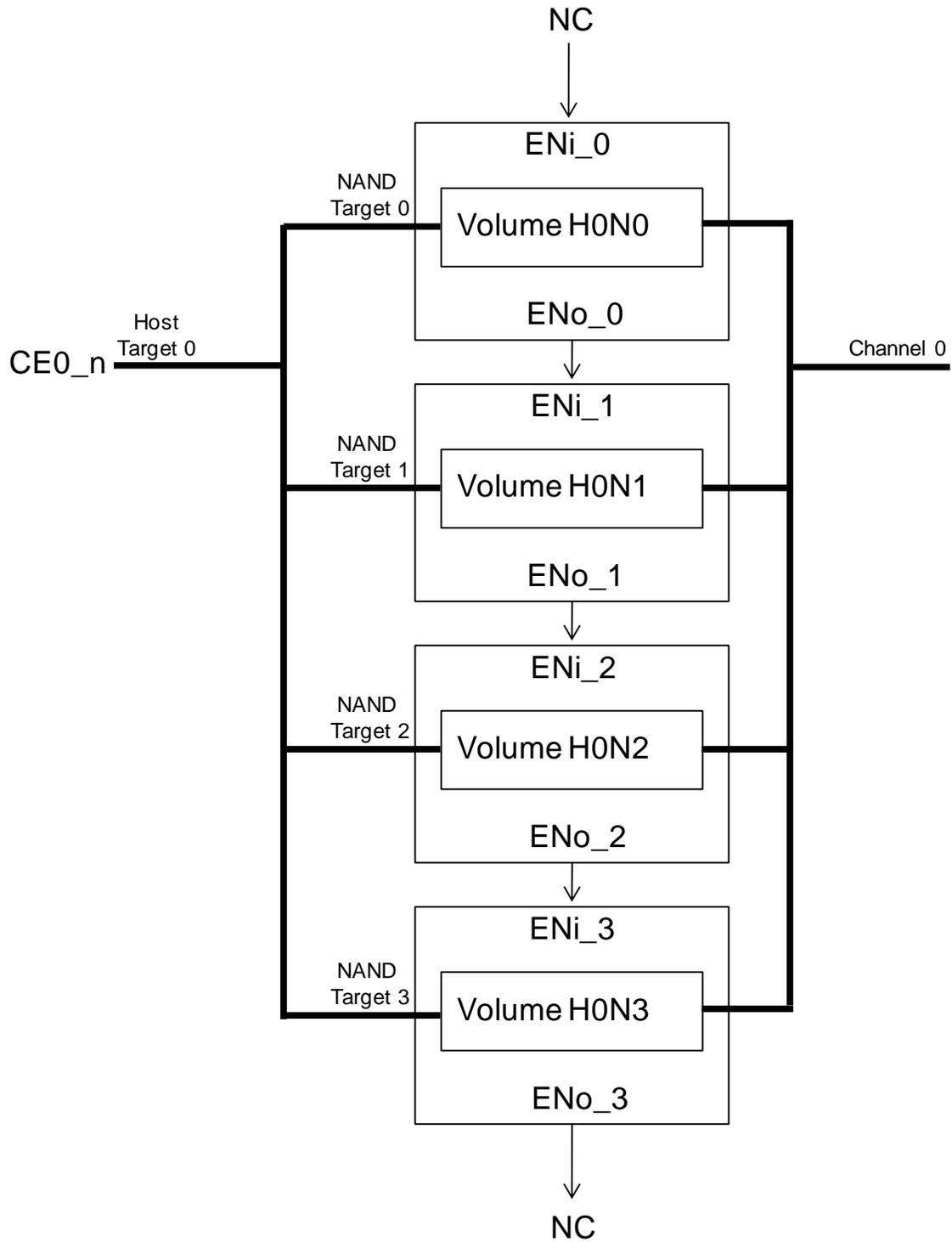
Figure 2-34 CE<sub>n</sub> Pin Reduction Topology, example 1
