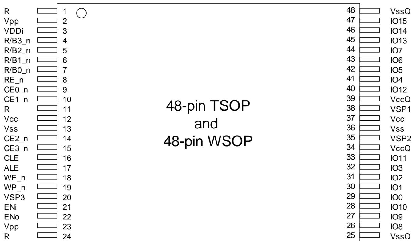
**Figure 2-2 48-pin TSOP/WSOP pinout for 16-bit data access**
