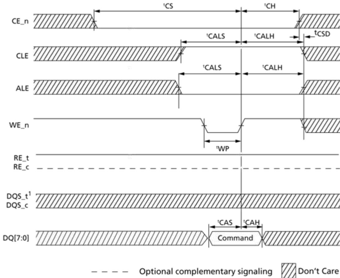
Figure 4-40 Command cycle timings
