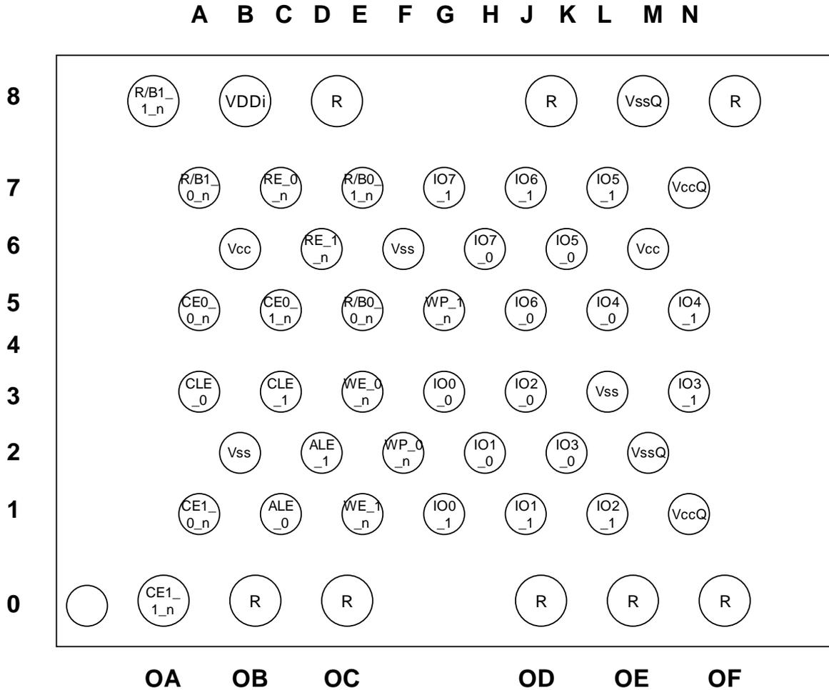
Figure 2-3 LGA pinout for 8-bit data access
