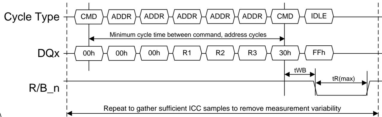
**Figure 7-1 ICC1 measurement procedure**
