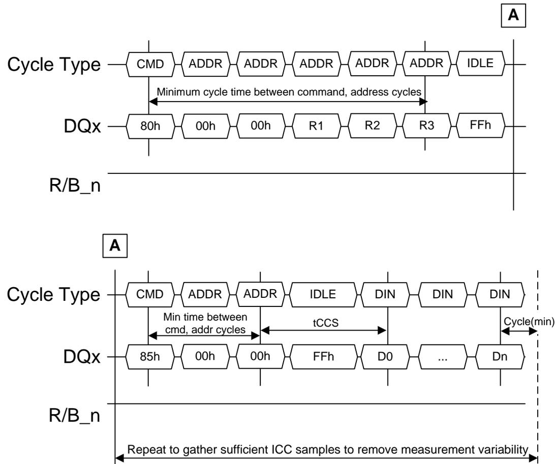
**Figure 7-5 ICC4W measurement procedure**
