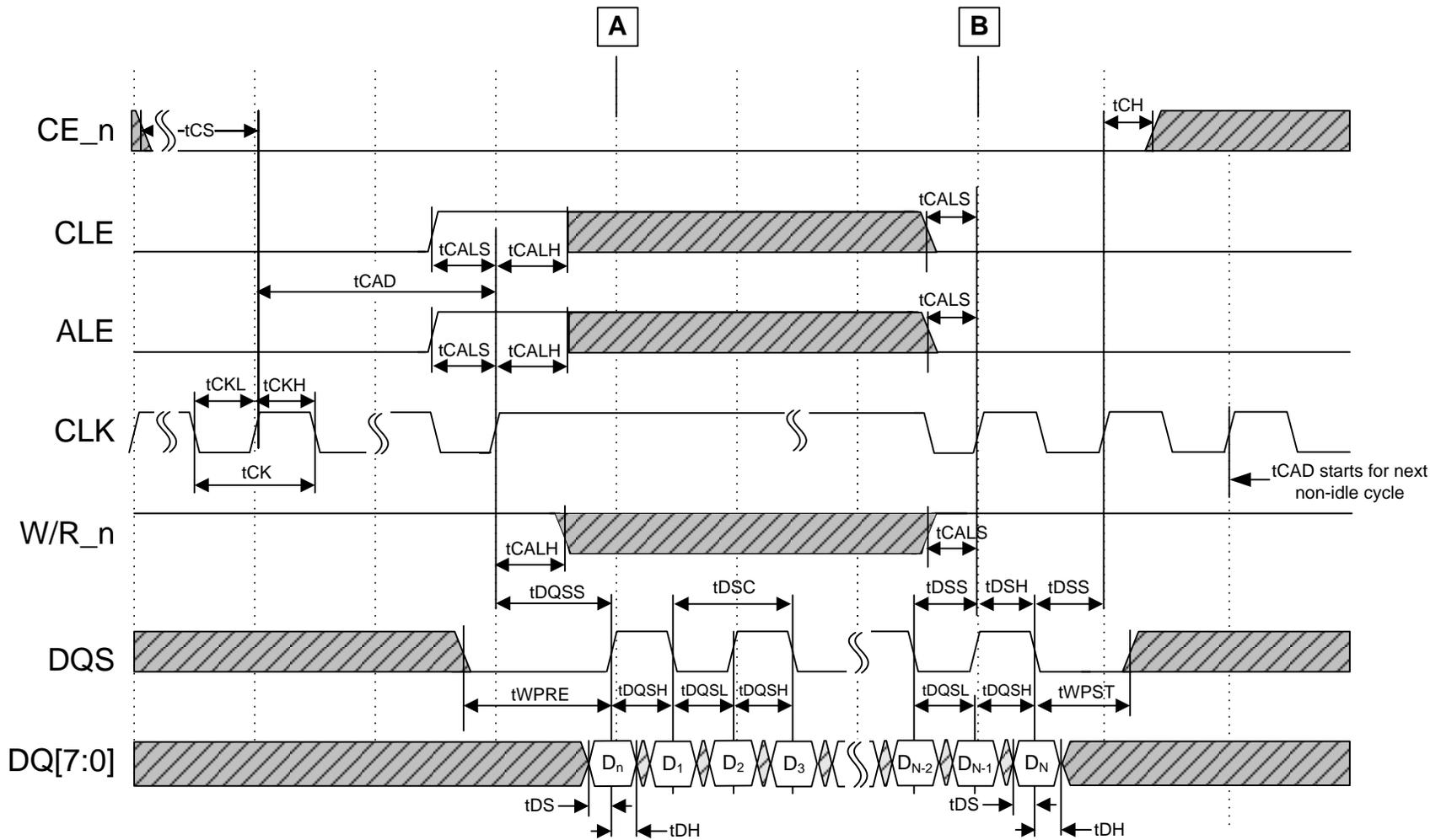
Figure 4-34 Data input cycle timing, CLK stopped
