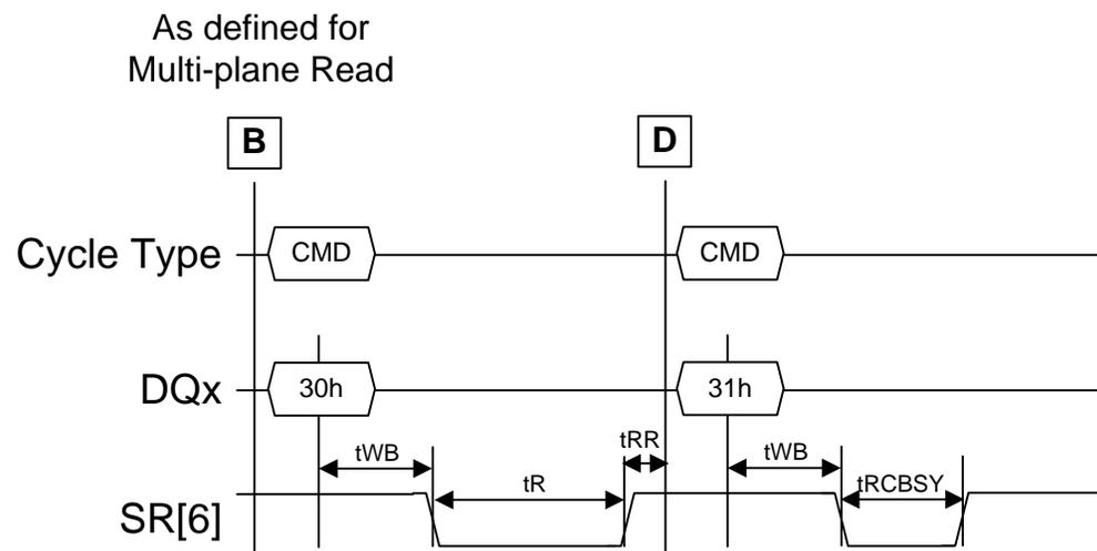
**Figure 6-12 Multi-plane Read Cache Sequential command issue timing**
