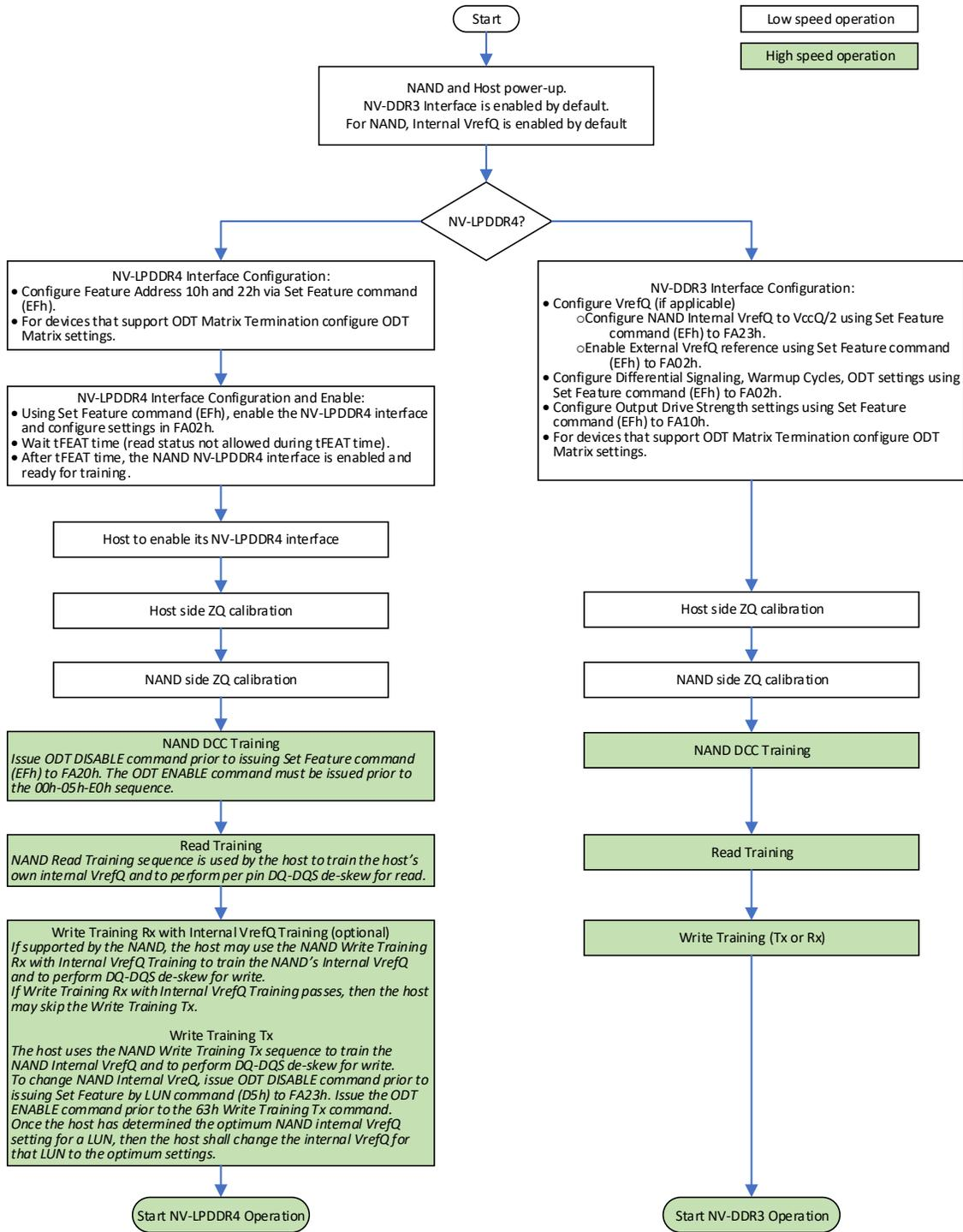
Figure 4-5 NV-DDR3/NV-LPDDR4 Initialization Flow
