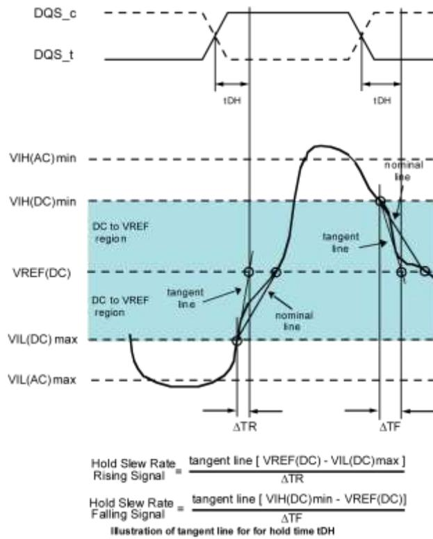
Figure 4-15 Tangent Line for Data Hold Time (tDH)
